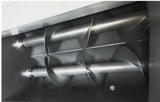
双螺杆设计,带特氟龙涂层。 Double-Screw Design, coated with Teflon.
